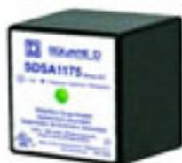
**To Test:** To test a Square D Surgebreaker Secondary Surge Arrester, look for the green LED indicator light on the front of the unit. If the light is on, the unit is operational. If not, the unit should be replaced. Always check the surge arrester after a storm to make sure it is still working.
