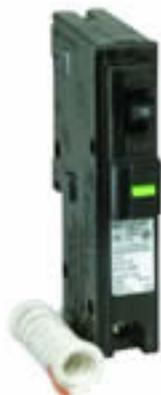
**To Test:** To test the Square D Arc-Fault Interrupter, turn OFF all loads downstream of the circuit breaker. Make sure power to the electrical panel is ON and the circuit breaker handle is in the ON position. Push the green test button on the circuit breaker. If the circuit breaker is operating correctly, it will trip, and the handle will move to the tripped (center) position. Remember to reset the AFI circuit breaker by moving the handle to the OFF position and then back to the ON position.
